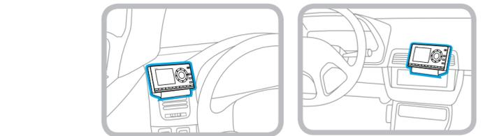
**B.** Some vents have recessed louvers. If yours are recessed, remove the regular vent clamps and install the extended vent clamps.
