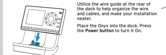
Utilize the wire guide at the rear of the dock to help organize the wire and cables, and make your installation neater.
