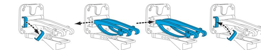
**C.** Attach the Vent Mount to the PowerConnect Vehicle Dock using the 4 provided screws.
