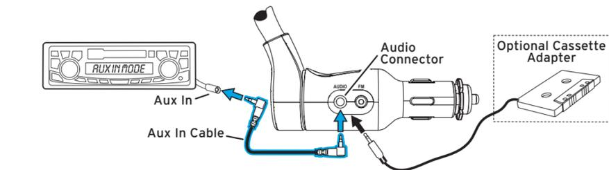
**TIP!** The auxiliary input jack may be located on the face plate of the vehicle radio, on the back of the radio, anywhere on the front dash panel, inside the glove compartment, or inside the center console in between the front seats.
