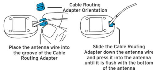
Place the antenna wire into the groove of the Cable Routing Adapter
