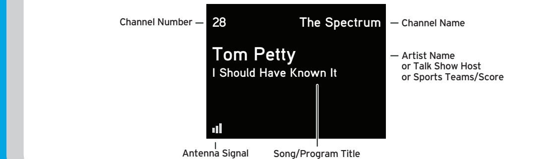
Channel Number — 28 — Channel Name The Spectrum — Artist Name or Talk Show Host or Sports Teams/Score Tom Petty — Song/Program Title or Talk Show Schedule or Game Time/Game Details I Should Have Known It — Antenna Signal Strength
