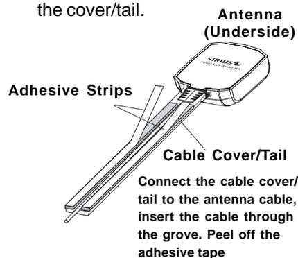
3. Remove the remaining protective tape from the adhesive, carefully position the antenna with cover/tail and apply pressure to secure to the vehicle.
