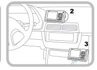
B. Orient the adhesive foot so that Roady BT is easily accessible. Loosen the knob and adjust the adhesive foot to position 1, 2, or 3, and then tighten it.
